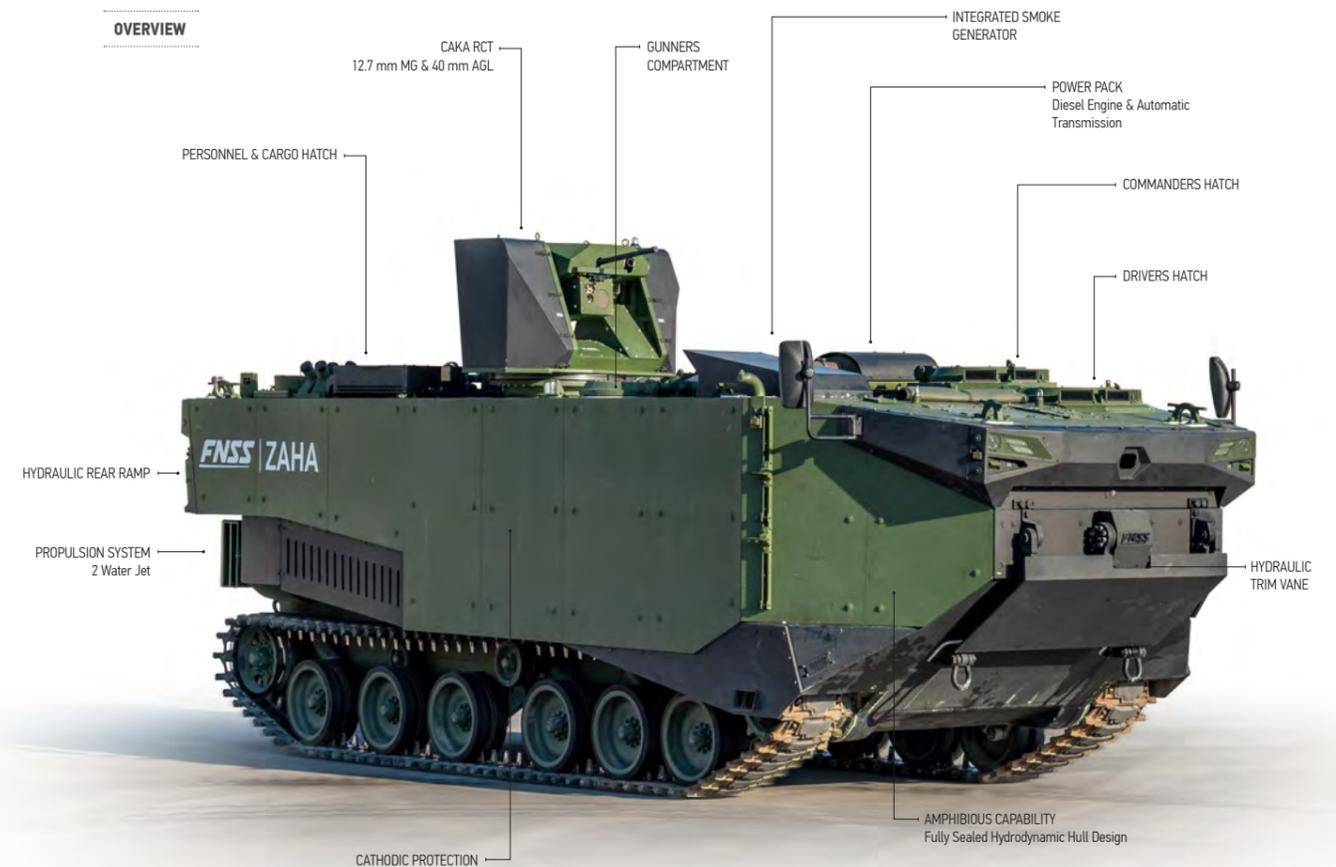
**During the beach-landing phase of amphibious operations, these vehicles are launched from amphibious assault ships and are able to rapidly cover the distance between the vessel and the shore, allowing marine units to land under armour protection. MAV have all the features and capabilities of both a military land vehicle and a military marine vessel, by balancing the land and sea requirements. This dual role by definition, vehicle offers high performance both on land and water operations.**
