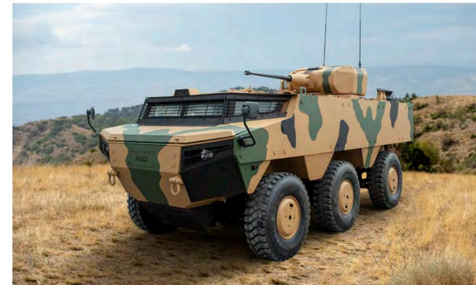
Under favour of hydro-pneumatic suspension system, the vehicle has the best road holding and ride height for different road conditions. PARS SCOUT 6x6's turning radius and the tire wear are minimized thanks to AWS (All Wheel Steering) System. PARS SCOUT 6x6 has a range of over 800 km, and it has under-armour protected fuel tanks. The vehicle is fitted with run-flat tires and with a self-recovery winch.
