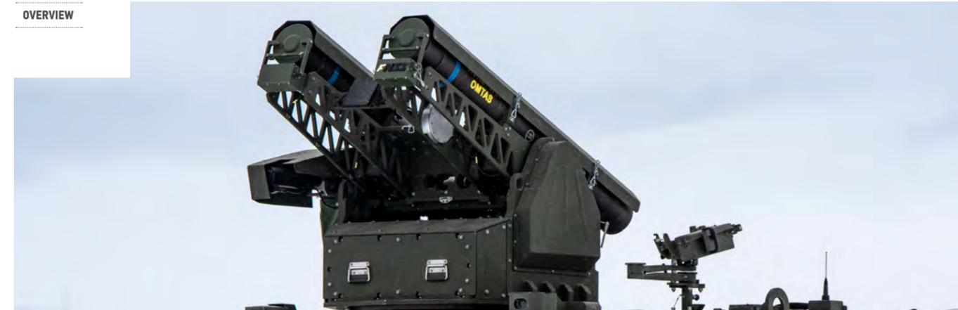
**The ARCT was designed specifically for the anti-tank role from the very outset and has some important integrated features that turrets with add-on missile capability are lacking. The ARCT offers the best optimization for low silhouette, armour protection, ergonomics, easy conversion to tripod launch configuration and sighting system.**
