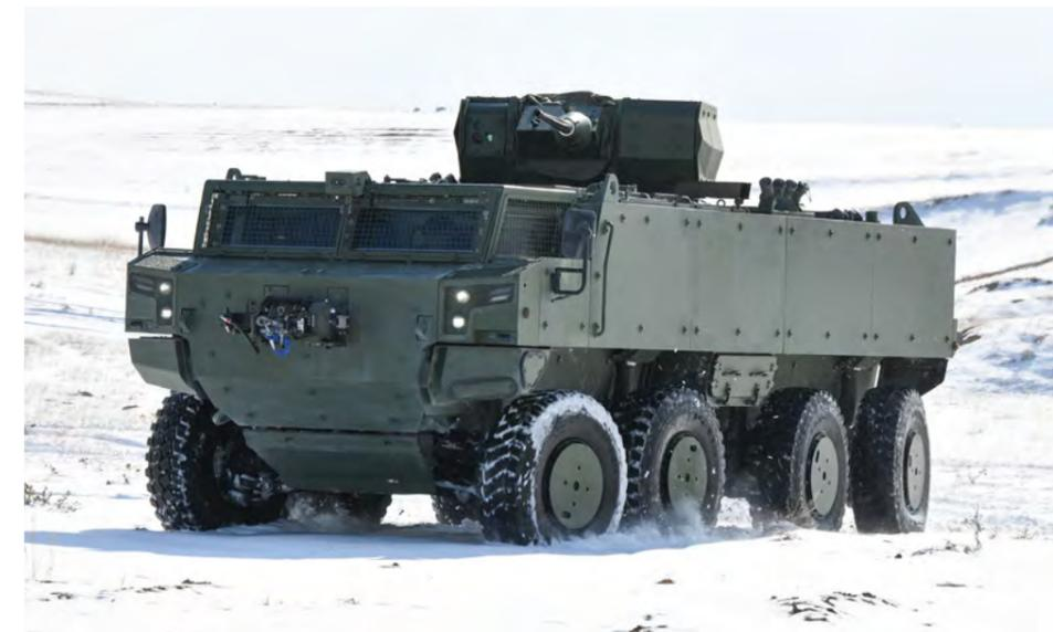
Under favour of hydro-pneumatic suspension system, the vehicle has the best road holding and ride height for different road conditions. PARS SCOUT 8x8's turning radius and the tire wear are minimized thanks to AWS (All Wheel Steering) System. PARS SCOUT 8x8 has a range of over 800 km, and it has under-armour protected fuel tanks. The vehicle is fitted with run-flat tires and with a self-recovery winch.
