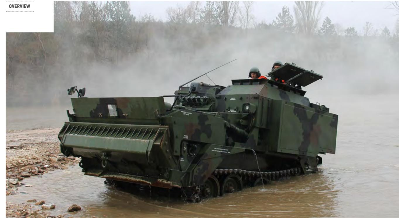
**The AACE is an amphibious, armoured, tracked, combat earthmover, designed for the preparation of river banks during river crossing missions. It is capable of performing bulldozing, rough grading, excavating, hauling, and scraping operations.**
