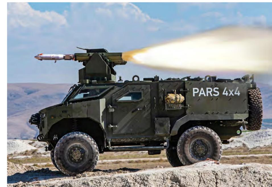
The driver's cabin features a transparent ballistic armour which offers a wide field of view for both the driver and the crew. The PARS 4x4 also provides the driver and the commander with integrated night and day vision cameras that enable operations in the dark with or without using blackout lights. The command and warning panels and the height-adjustable mine-protected seats have been specifically developed for the commander, driver, gunner and dismounts.
