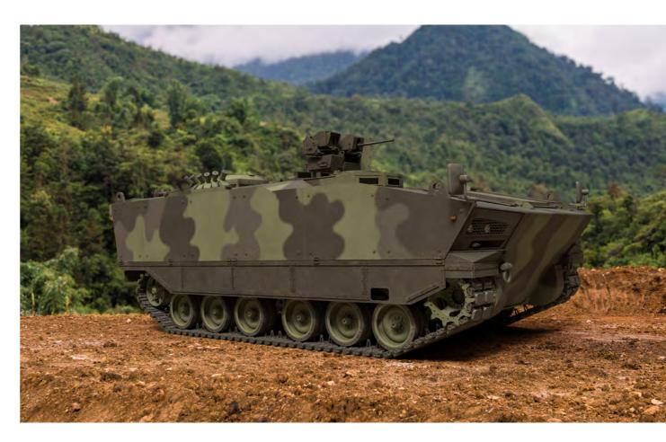
KAPLAN APC is a modular vehicle, designed with possible integration options for manned and unmanned turret systems, armed with light and medium calibres as well as 120mm mortars and ATGM turrets and weapon systems.
