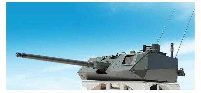
SuperShot 40 mm (40x180 mm) ammunition can also be used in the turret as the 30 mm cannon can be easily converted by a simple replacement on the field to fire those 40 mm rounds.
