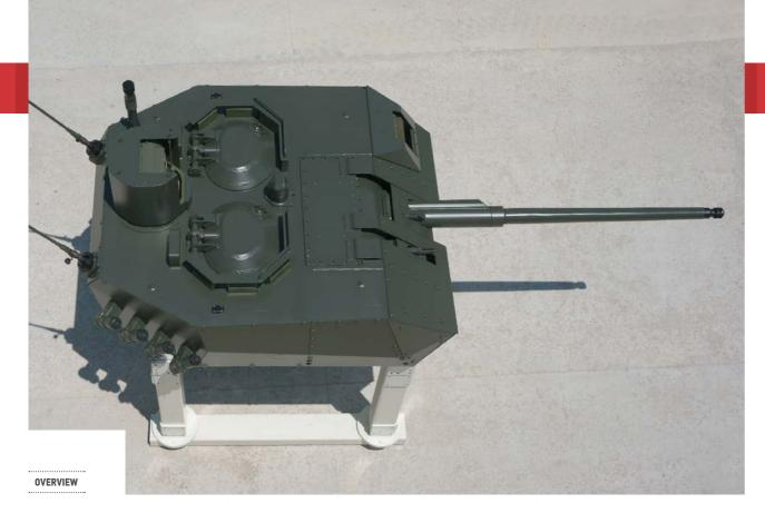
The TEBER-30 Two-Man Turret, is a medium caliber turret that can be fitted to wheeled and tracked armoured vehicles and is offered in two configurations. In the conventional two-man configuration, the commander and the gunner are positioned in the turret basket.
