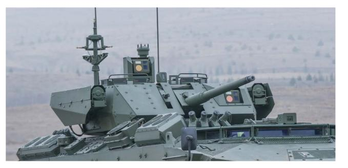
Two each ATGM missiles are integrated to both sides of the turret. According to user requirements, various modern anti-armour systems (ATGM's) such as Semi-automatic command to line of sight (SACLOS) and Automatic command to line of sight (ACLOS) guided missile can be integrated on turret's modular ATGM launcher. Two ATGM launchers can be operated seperately as well giving the user to opportunity to elevate at different angles to fulfill requirements of most common ATGM missiles on the market.
