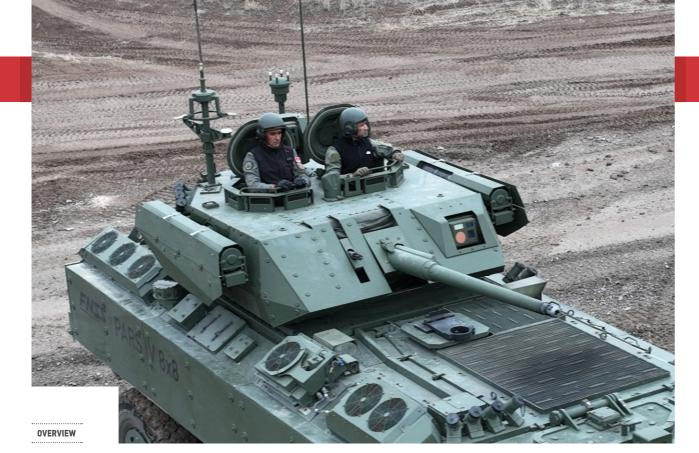
The TEBER-II 30/40 TMT (Two-Man Turret), is a medium caliber turret that can be fitted to wheeled and tracked armoured vehicles and is offered in two configurations. In the conventional two-man configuration, the commander and the gunner are positioned in the turret basket.
